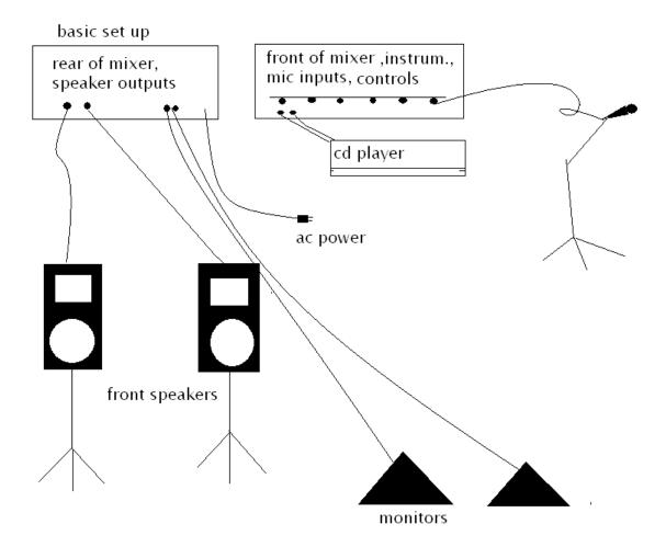
Make sure the "signal path" is logical. Follow from sound source (voice, instrument, CD) through to the speakers.
