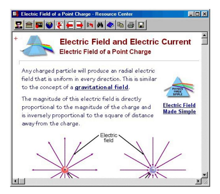
Here is an example of the electric field of a point charge:
