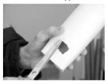
**Step 2**: Cut slits in the sides of the milk carton to hold the mirrors. The angle and location of the mirror will have an impact on making the periscope work.
