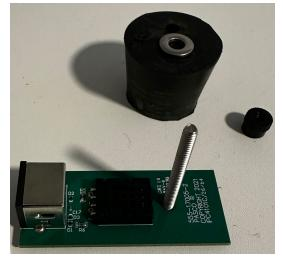
4. Place the temperature / humidity sensor board inside of the top piece of the Ecochamber underneath one of the holes. Push the 2-holed stopper through the top of the hole of the Ecochamber feeding the long screw up through the stopper. Secure the board to the stopper using the provided screw and washer. *It may be helpful to preconnect the temperature / humidity board to its cable before securing it to the stopper.*
