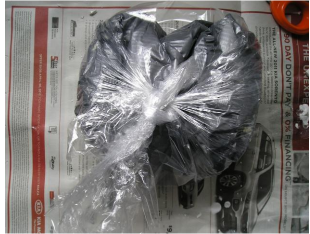
Saran wrap pulls the form into a more rounded shape and is tied in behind to hold it in place (only if the form needs to be more curved.)
